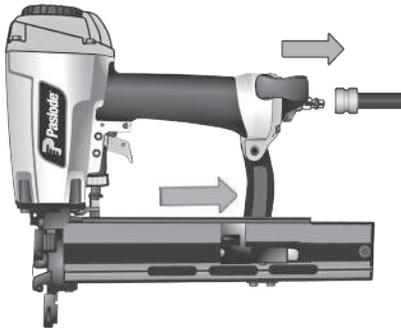
**Step No. 2** – Insert the staple strip into the magazine rail.
