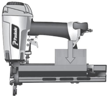
**Step No. 3** – Press the follower latch release lever or unlatch the follower and slide the follower forward until it contacts the staple strip. Reconnect air supply. The tool is now ready for use.
