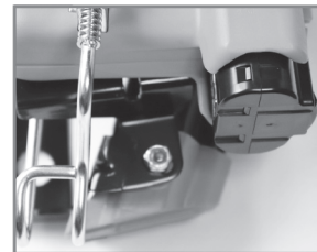
Remove nut from rear of magazine.
