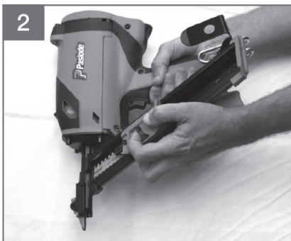
Depress lever, then pull nail follower back past nail strip
