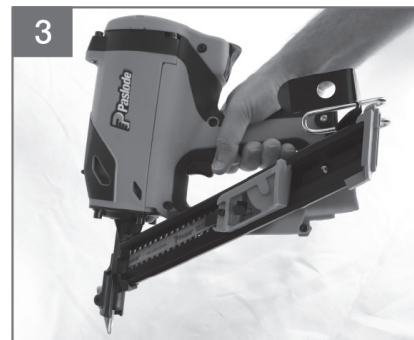
Gently release follower onto rear of nail strip, to prevent collation damage
