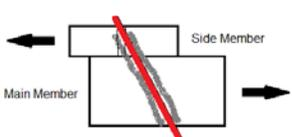
$Z = \frac{k_1 D l_s F_{es}}{R_d}$      | <p>For <b>Mode IV</b></p>
