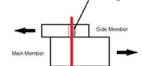
$Z = \frac{Dl_s F_{es}}{R_d}$ | <p>For <b>Mode III<sub>s</sub></b></p>
