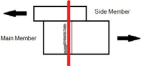
$Z = \frac{Dl_m F_{em}}{R_d}$ | <p>For <b>Mode III<sub>m</sub></b></p>
