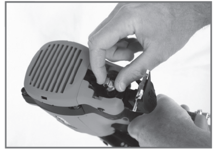
Carefully align fuel adaptor and cell stem
