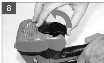
8 Note: Fuel cell Dosing Lever must be in the down position
