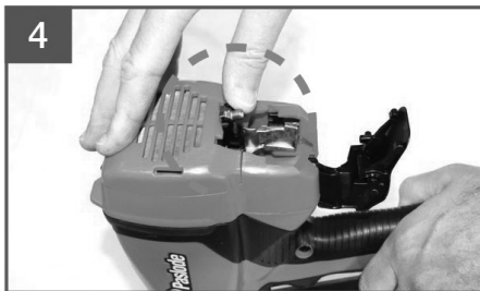
4 Raise fuel tube block assembly, it will lock in up position
