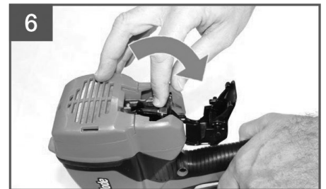
6 Carefully align fuel adaptor and cell stem
