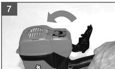
7 To close - Push forward, then down to lock fuel door
