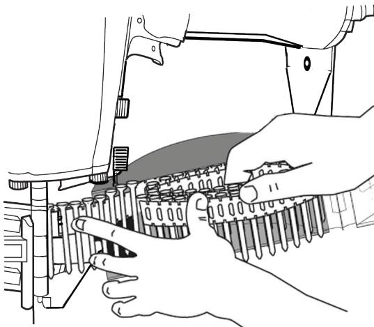
Step No. 3- Slide the free strip of nails along the top of the feeder body assembly and feed the nails over the feed pawls until the first nail is in the nose raceway.
