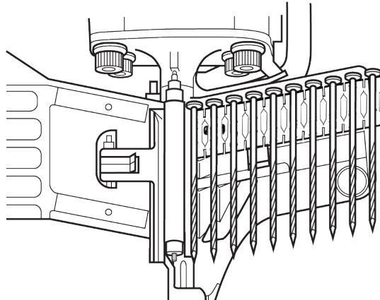
Step No. 4- Close the magazine cover and then the gate making sure the gate is latched securely.
