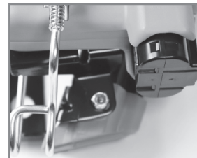
Remove nut from rear of magazine.
