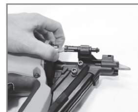
Reassemble tool, attach magazine to nose, replace cap screws and nut. Tool is ready to use.
